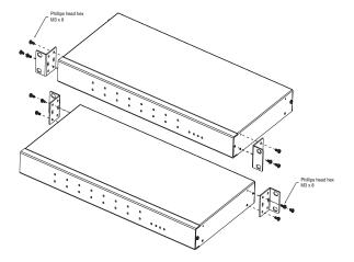
3. Slide the unit into the front or rear of the rack and secure it to the rack.
